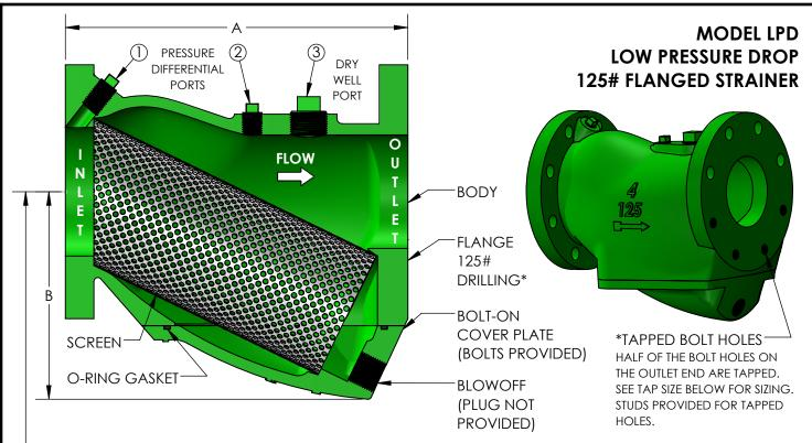
C (CLEARANCE TO REMOVE STRAINER FROM BELOW) \*IF THERE IS NOT ENOUGH CLEARANCE BELOW STRAINER, PRODUCT CAN BE ROTATED 90° AXIALLY TO PROVIDE CLEARANCE OR FOR STEAM APPLICATION TO MINIMIZE CONDENSATE COLLECTION
