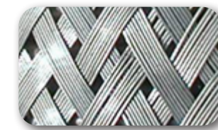
Single braid is made up of groups of wires called carriers or bands.
